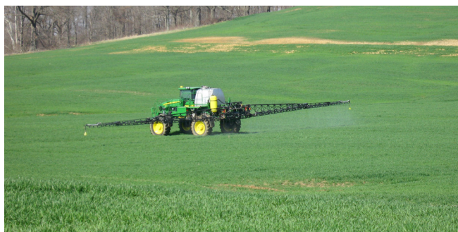
Photo 5-7. Most nitrogen fertilizer is applied as a liquid urea ammonium nitrate (UAN) and 28% or 32% N. By using stream bars or stream jet style nozzles, leaf burn from UAN is minimized.
